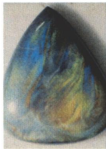
Fig. 12. Photograph of a pear shaped cabochon cut dark Russian synthetic opal showing a wavy, fibrous, paintbrush pattern of very small colour grains.
