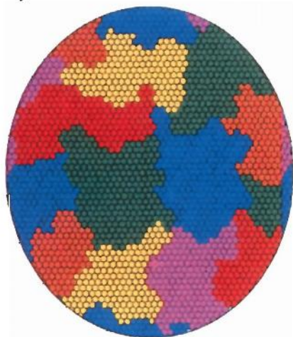
Fig. 18. Diagram of the 'lizard skin' effect seen in 'synthetic' and 'imitation' opals.
