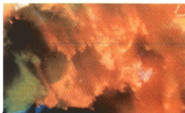
Fig. 22. Characteristic 'dangling stalactitic' colour distribution in a Gilson manufactured fire opal (imitation). Oblique lighting. 40x, Reproduced (with permission) from figure 8 of Gundawardene, M. & Mertens, R. (1984) Gilson created fire opal imitation with play of colours. Journal of Gemmology . 19(1), 43-53.
