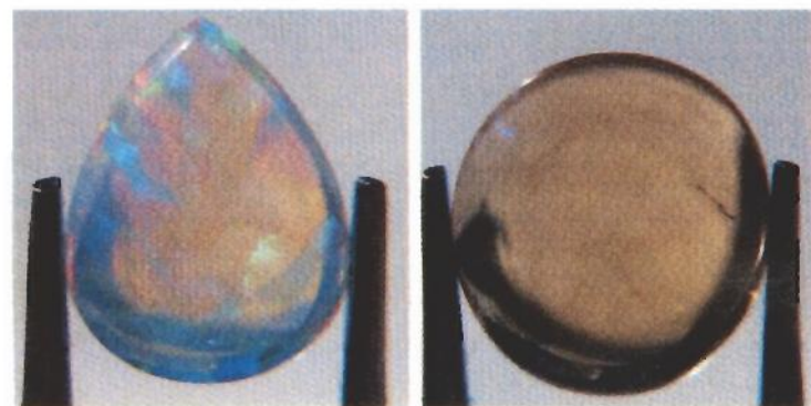
Fig. 7. Photograph in transmitted light showing a comparison of a natural light opal oval cabochon and a pear shaped 'synthetic' opal cabochon, note the yellowish colour of the natural opal when compared to the pinkish colour of the 'synthetic' opal.
